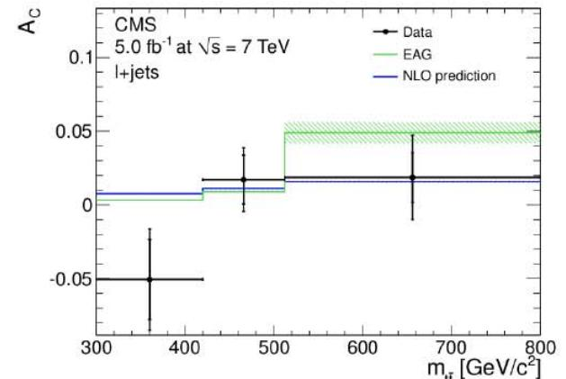
Asymmetry measured in  $p_T$ ,  $y$  or invariant mass of the top pair system
